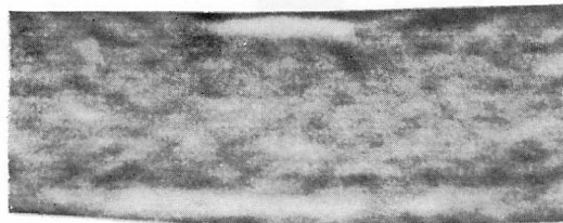
Fig. 8. Influence of the carrier-frequency of the transducer on the texture of echocardiographic phantom images.
