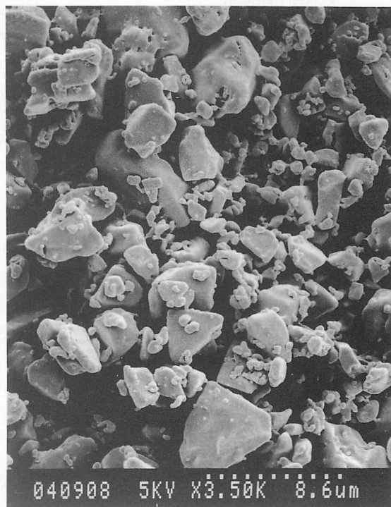
Fig. 1 Microscopic view of the surface of one granule of SH/TA-508 (magnification \times 3,500 )
